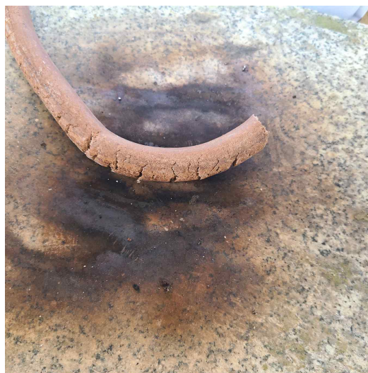
Figure 6.2 Pellet with crack
